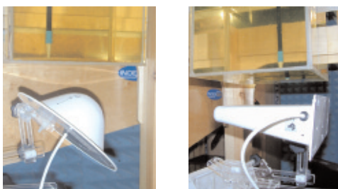
Compliant Body SAR Test Measurement System Small Base Station Antennae test set-up shown
